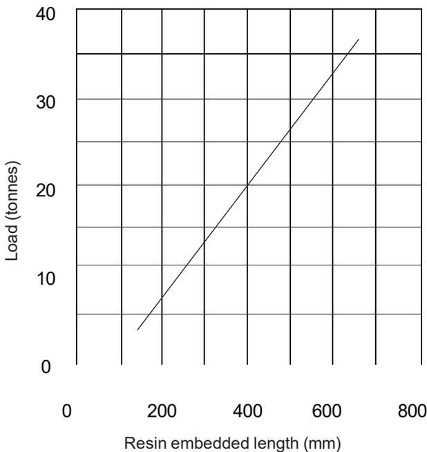
Note: The graph illustrates typical failure loads. Minimum safety factors of 1.5 in non-critical and 2 in critical cases should be considered for design purposes. Where relevant, the local codes of practice or standards must also be considered in relation to anchorage length.
