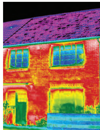
Substantial heat loss can occur through single skin walls. Photo courtesy of iRed Ltd
