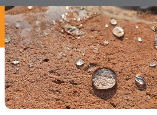
**DrySeal** is a, unique, thixotropic, water repelling masonry protection cream which can be used on a range of building materials. Dependent on the porosity of the substrate, the effective siloxane ingredient penetrates the substrate within a short period of time (30 minutes to several hours), where it reacts to become a permanent, chemically bonded, silicone coating.
